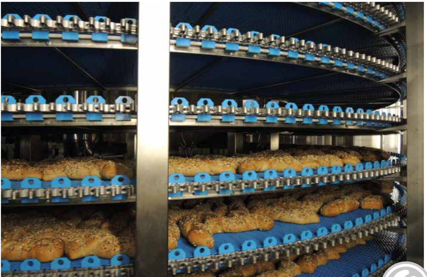
Air-forced room cooling
