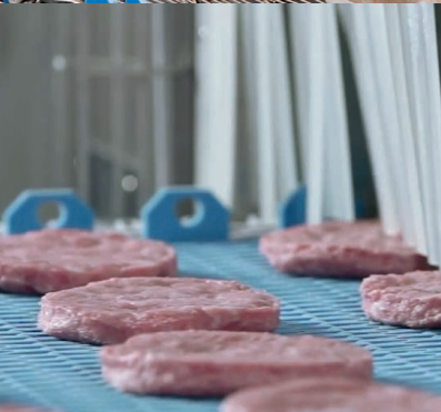
Plastic mesh open area from 55% to 84%
